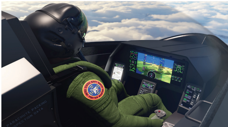
Figure 1 - The Collins Aerospace Advanced Flight Deck - utilizing a Modular Open Systems Approach (MOSA) to rapidly deploy new technology upgrades when needed to overcome the latest threats
